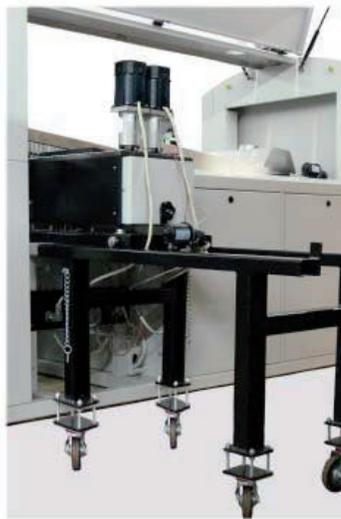
*Motorized roll-out pot (optional) provides easy access.*
