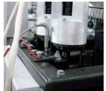
*Solder level sensor with alarm*
