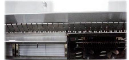
*Independently controlled infrared and forced air convection preheaters compatible with VOC-free fluxes.*
