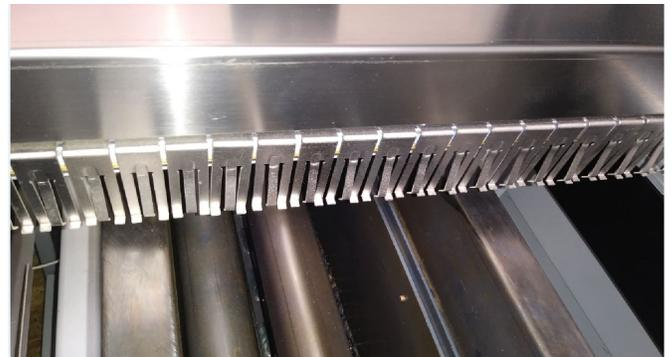
*Finger conveyor for pallet or pallet-less operation.*
