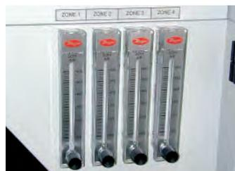
Novastar's isolated chamber design (recirculation of atmosphere within each chamber) maintains low oxygen levels while conserving nitrogen.
