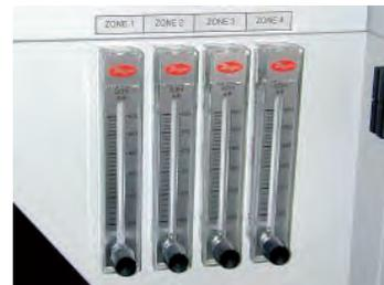
All GF ovens have a nitrogen gas inerting option. With the isolated chamber design (recirculation of atmosphere within reflow zone) low oxygen levels are maintained while conserving nitrogen consumption.
