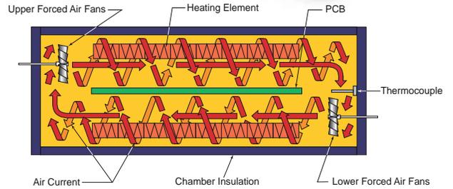
Our patented Horizontal Convection™ technology\*\* circulates heated air in each chamber around the board front to back which increases the thermal efficiency and uniformity within each zone. This exposes the circuit board to a uniform temperature profile along the entire assembly. Cyclonic generator speed is independently set in each zone.
