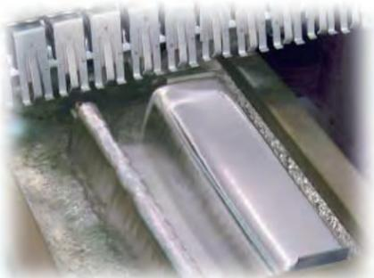
Turbulent wave for SMD and laminar wave for through-hole soldering
